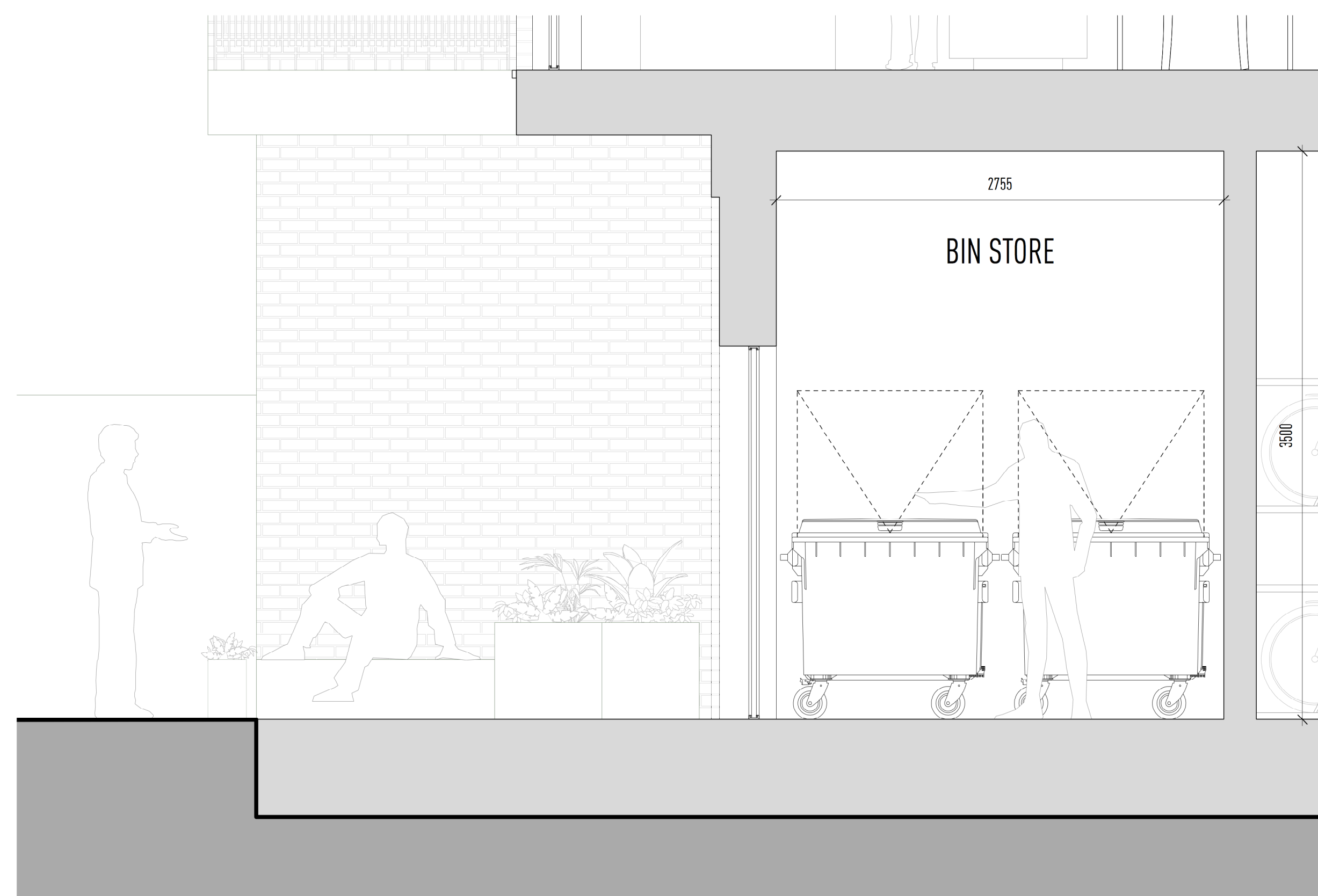
03 - Proposed Bin Storage Section (Bin Store 3) 1:25@A1
